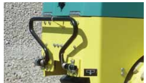
Optional safety bar with simple transport lock
