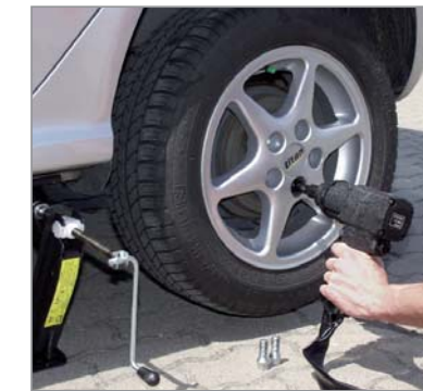
Impact wrenching for fast wheel changes
